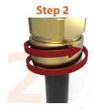
Tighten backnut until a seal is formed onto the cable, then tighten one further turn
